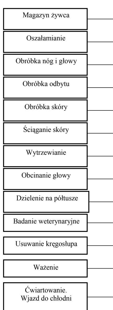
Rys. 1. Schemat procesu technologicznego uboju i obróbki bydła Fig. 1. Figure of the technological process of slaughter and processing of cattle
