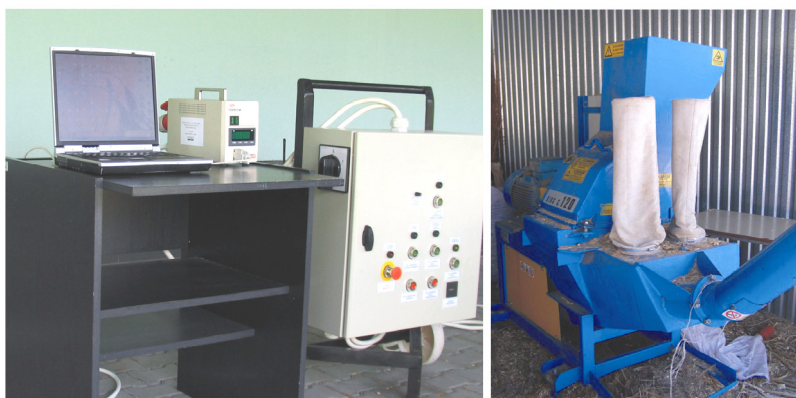
Rys. 4. Stanowisko do badań energochłonności mielenia materiałów roślinnych [fot. K. Mudryk] Fig. 4. Workstation for the analysis of energy consumption in the process of grinding of vegetable materials [photo by K. Mudryk]
