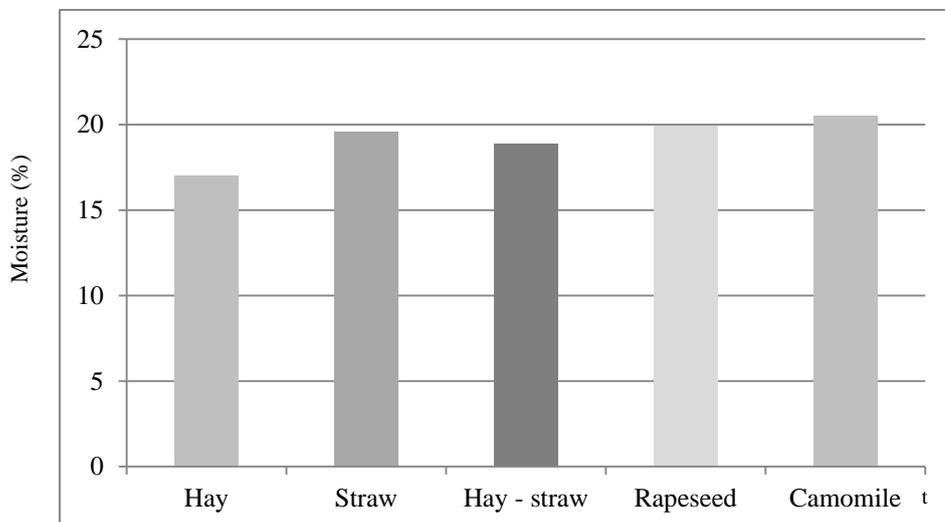
Figure 3. Average moisture of particular raw materials supplied to the plant
