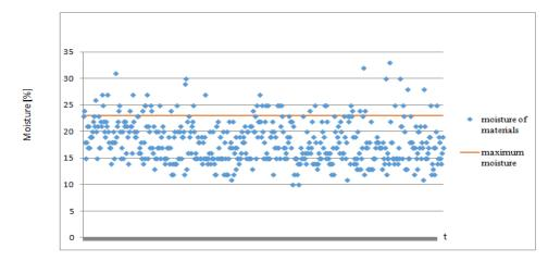
Figure 2. Moisture of raw materials supplied to the pellet plant with designation of the maximum (assumed by the pellet plant) moisture of raw material designed for production
