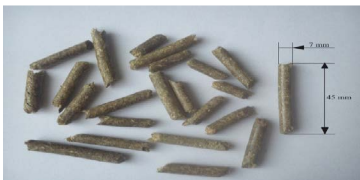
Figure 2. Fuel pellet produced in the pellet production plant
