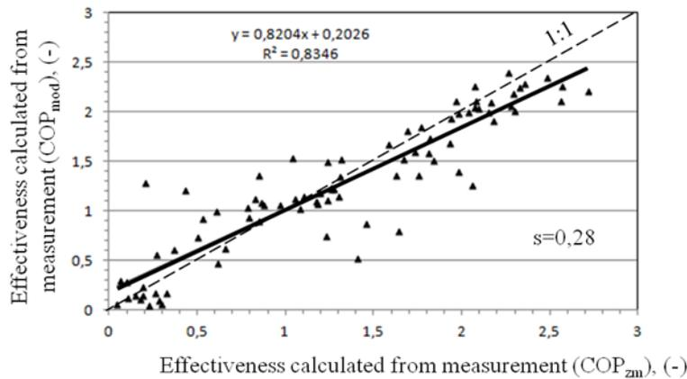
Figure 5. Comparison between the calculated and measured values of COP
