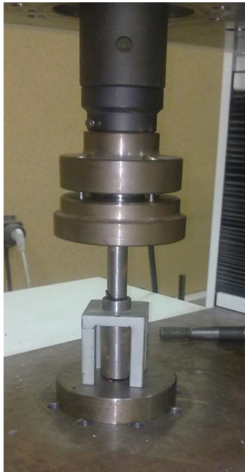
Figure 3. Simplified Pelletizing Test Apparatus
