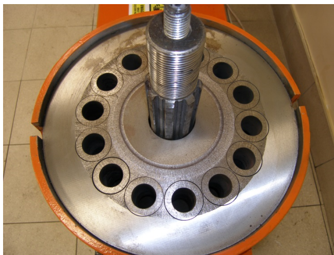
Figure 2. Briquetting matrix with diameter of meshes of 28 mm and length of meshes (sleeves) 80 mm
