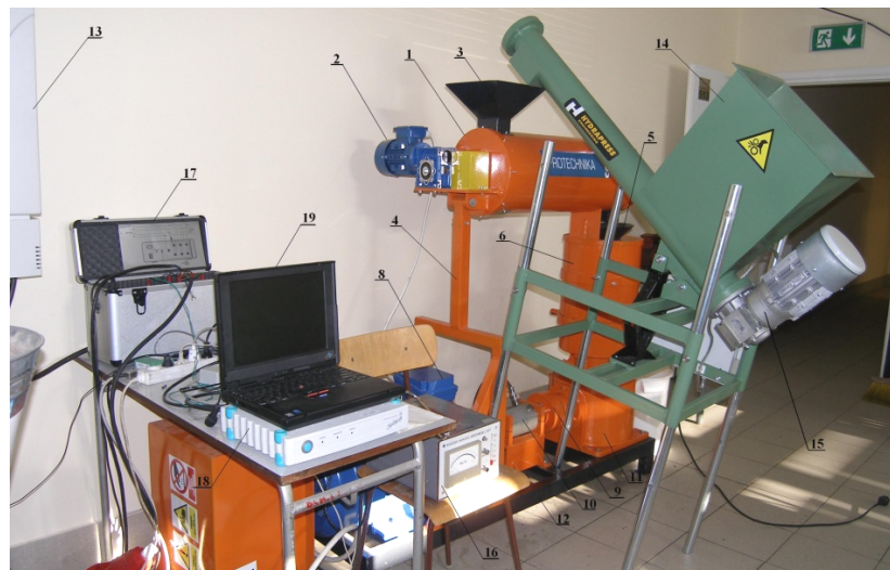
Figure 1. Test rigs with new prototype densifying-briquetting device with a flat immovable matrix: a) scheme of test rigs: 1 – mixing–densifying–dosing system, 2 – drive of mixing–densifying–dosing drive (electric engine connected to reducer), 3 – feed of raw material to mixing–densifying–dosing system, 4 – mounting frame for mixing–densifying–dosing system, 5 – batch of initially compacted raw material to working system of pelletizer, 6 – working system of pelletizer, 7 – discharge of pellets from working system, 8 – drive of pelletizer (electric engine), 9 – clutch, 10 – measuring torque Mi20, 11 – toothed gear, 12 – base, 13 – frequency converter, 14 – batcher, 15 – drive of batcher (electric engine connected to reducer), 16 – index of rotational moment and force WT-1, 17 – device for measuring active power METROL KWS 1083, 18 – recorder Spider 8, 19 – PC computer b) view of test rigs
