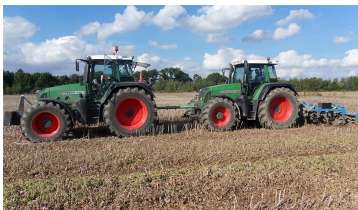
Figure 1. Measurement of the working resistance of a unit with a pulling method
