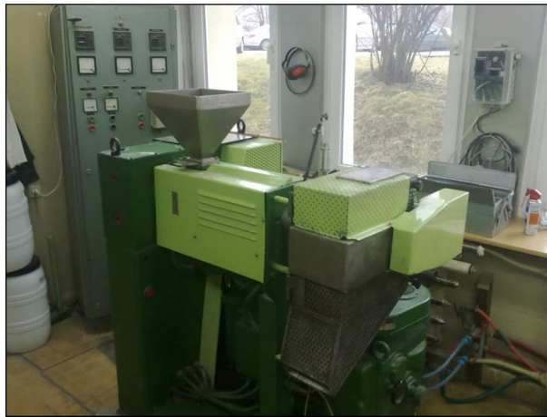
Figure 2. Single-screw extruder-cooker TS-45 with L/D=12
