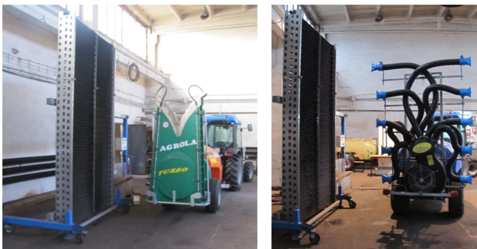
Figure 1. Sprayers used at the test rigs at the vertical droplet separator (patternator): horizontal emission system sprayer AGROLA Turbo 100v (left hand) and air directed emission system sprayer Tifone 1000 (right hand)
