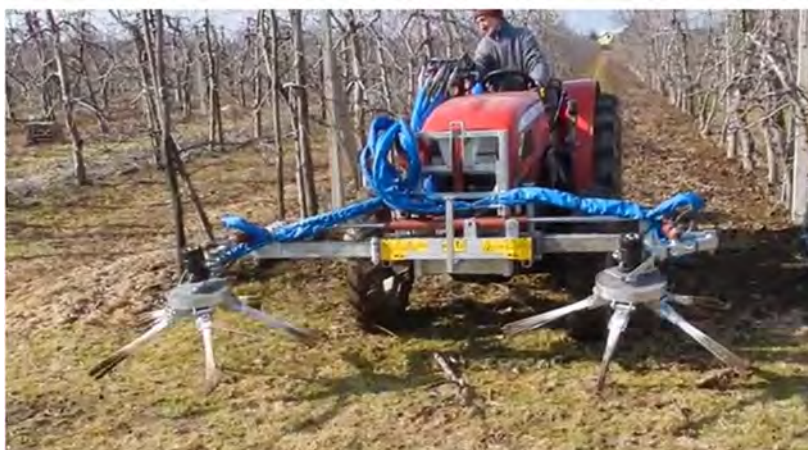
Figure 7. Sweepers gathering the pruned pulp into the middle of the interrow: a) with raking out elements, b) with belts
