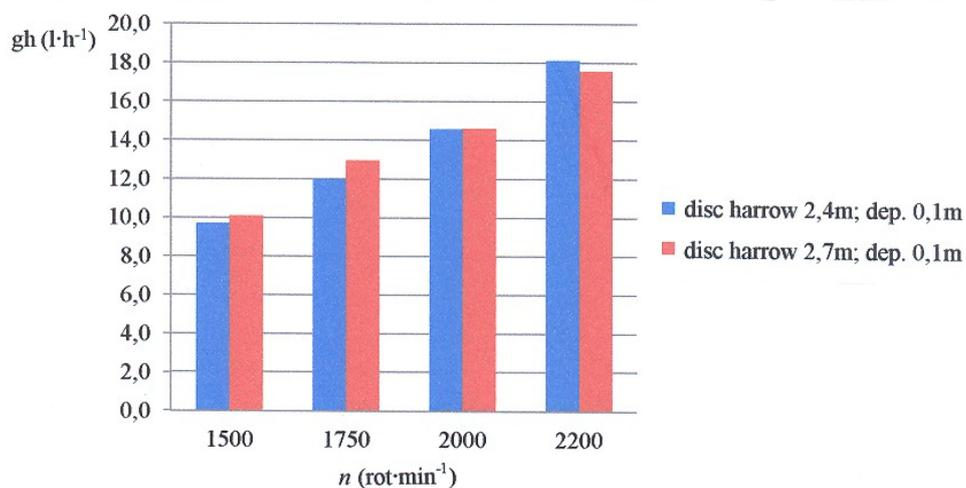
Figure 4. Relation of an hour fuel consumption for a tractor to rotational speed of its engine for disc harrows.  $g_h$  – hour fuel consumption,  $n$  – engine rotations
