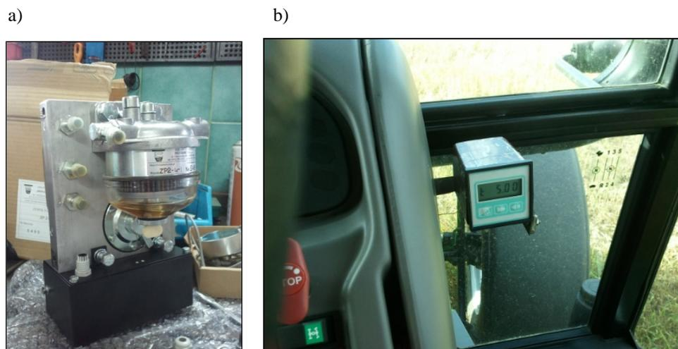
Figure 1. Measurement unit a – flow meter ZP@-4-I by Rotameter company, b – NOSAL-TECH mounted on a tractor
