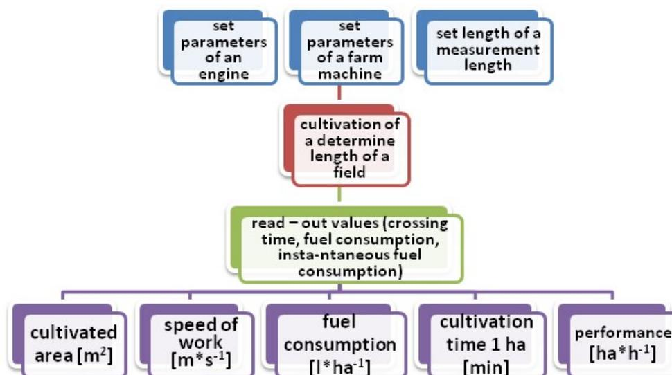
Figure 2. Schematic representation of procedure during exploitation tests
