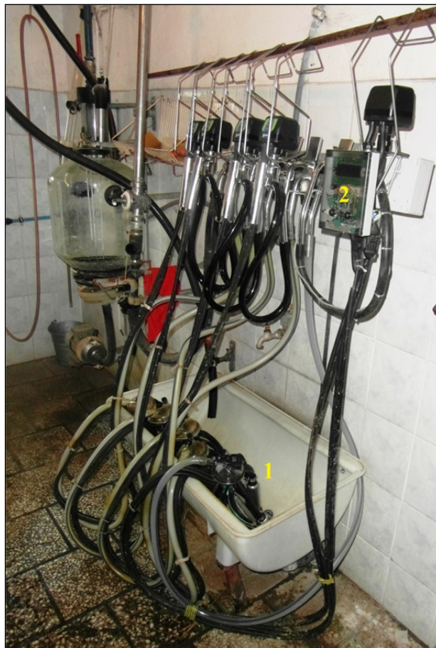
Figure 1. Milking device used in cowshed tests: 1 – milking apparatus with embodied thermistors 2 – microprocessor recorder of measurement signals
