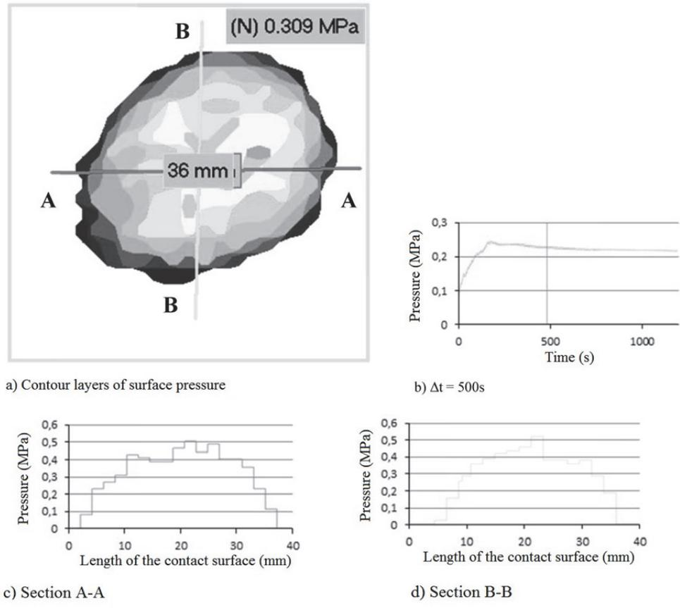
Figure 6. Contour layers and distribution of surface pressures in time  $\Delta t=500$  s
