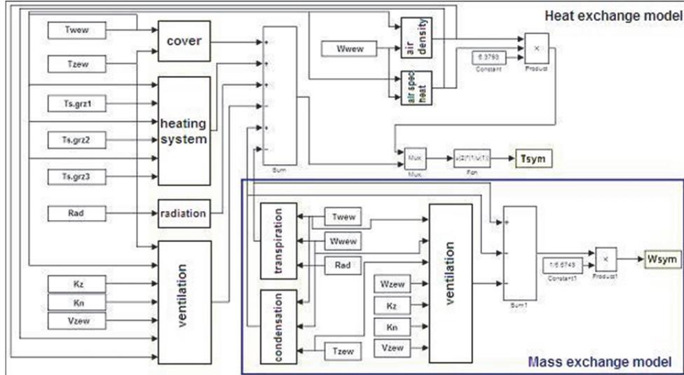
Figure 1. Schematic representation of the computer model of heat and mass exchange in air inside greenhouse. Symbols:  $W_{wew}$  – relative humidity of air inside greenhouse (%),  $W_{zew}$  – relative humidity of air inside greenhouse (%),  $T_{sym}$  – air temperature inside greenhouse obtained as a result of computer simulations ( $^{\circ}C$ ),  $W_{sym}$  – humidity of air inside greenhouse obtained as a result of computer simulations ( $kg_{pary} \cdot m^{-3}_{powietrza}$ )
