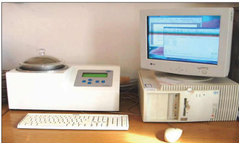
Figure 2. Laboratory pneumatic separator LPS 200 MC
