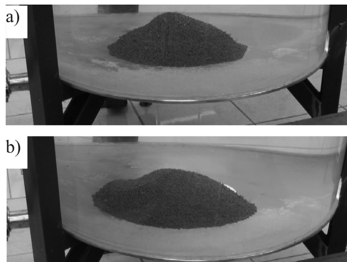
Figure 2. The final phase of forming the cone of sediment break (a formed cone of break - the end of cycling) next to the laboratory vat tilted to the inlet at: a) 2°; b) 6°
