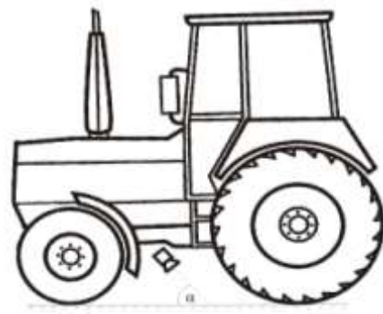
Fig. 3. Illustration of angle measurement for radar position relative to the ground
