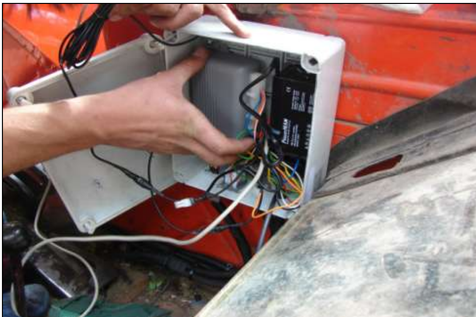
Fig. 4. Fitting of the vehicle on-board computer with UPS module - installed permanently in tractor cab
