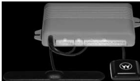
Fig. 2. Vehicle on-board computer (ET-GSM-GPS) with antennas: GSM antenna to the left, GPS antenna to the right
